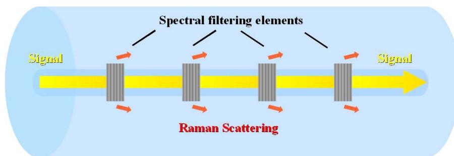
Figure 2. Fiber spectral filtering elements mitigate stimulated Raman scattering by removing the Raman scattered light from the fiber core.
