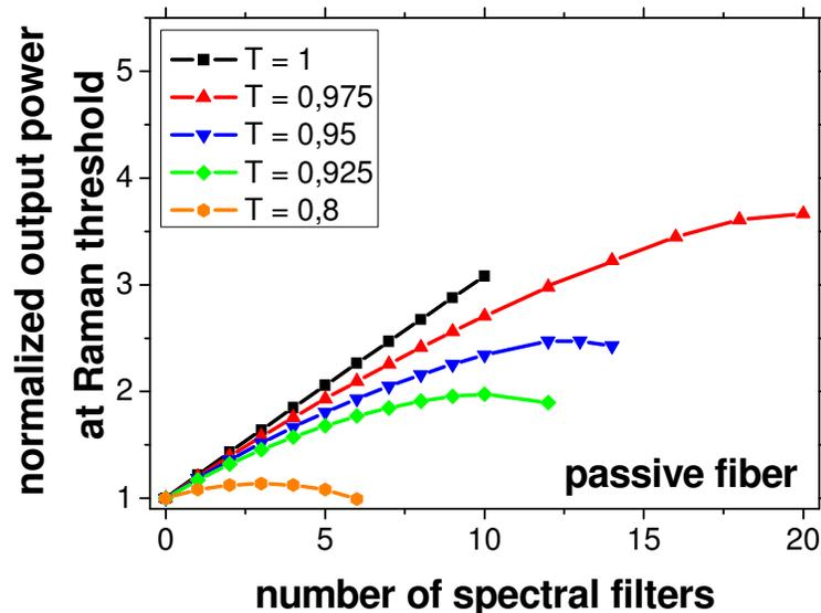
Figure 3. Simulated output signal power of a passive fiber at the Raman threshold normalized to the corresponding value for a fiber without spectral filtering. T denotes the filter transmittance at the signal wavelength.
