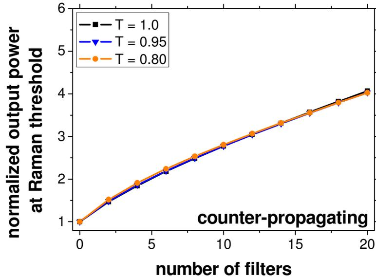
Figure 5. Simulated output signal power at the Raman threshold normalized to the corresponding value for a fiber without spectral filtering. T denotes the filter transmittance at the signal wavelength: For a counter-propagating amplifier and 20dB average Raman attenuation per filter.
