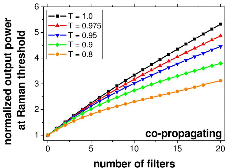
Figure 4. Simulated output signal power at the Raman threshold normalized to the corresponding value for a fiber without spectral filtering. T denotes the filter transmittance at the signal wavelength: For a co-propagating amplifier and 20dB average Raman attenuation per filter.
