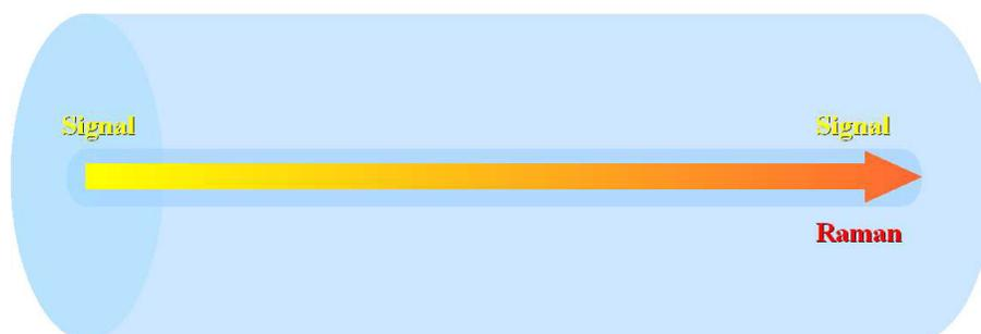
Figure 1. Stimulated Raman scattering transfers energy to longer wavelength when a certain threshold is reached.
