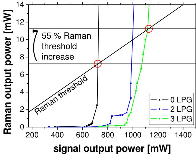
Figure 7. Raman output power vs. signal output power for three fiber configurations. Implementing long period gratings into the fiber increases the Raman threshold.
