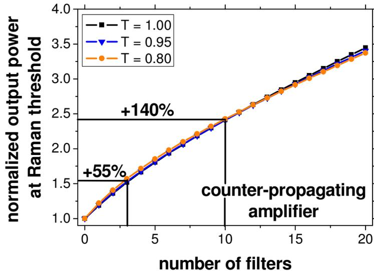
Figure 6. Simulated output signal power at the Raman threshold normalized to the corresponding value for a fiber without spectral filtering.  $T$  denotes the filter transmittance at the signal wavelength: For a counter-propagating amplifier and 15 dB average Raman attenuation per filter.
